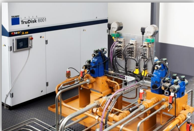
TRUMPF laser source powering the HYBWELDCUT demonstrator
